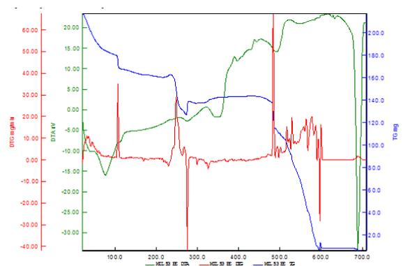
Fig. 6: DTA/TGA curves for MIL-53(Fe)
