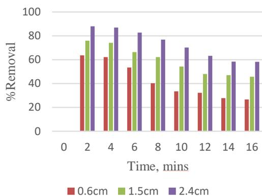
Fig.12: Bed height effect on adsorption of chromium
