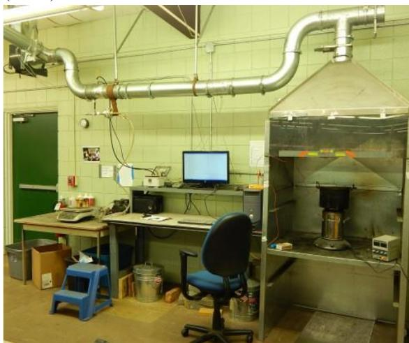
**Figure 2 Laboratory Emissions Monitoring System (LEMS)**
