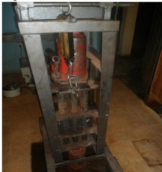
**Figure 1. Locally Fabricated Hydraulic Press Briquette Machine**
