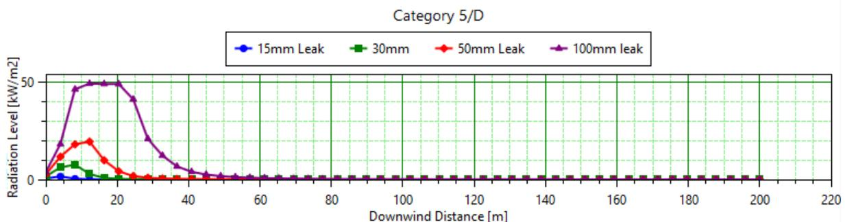
Figure 3: Radiation vs Distance for Jet fire
