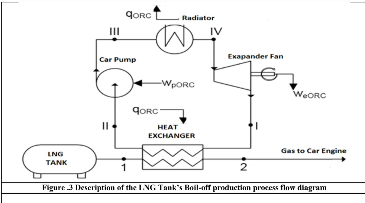
Figure .3 Description of the LNG Tank's Boil-off production process flow diagram
