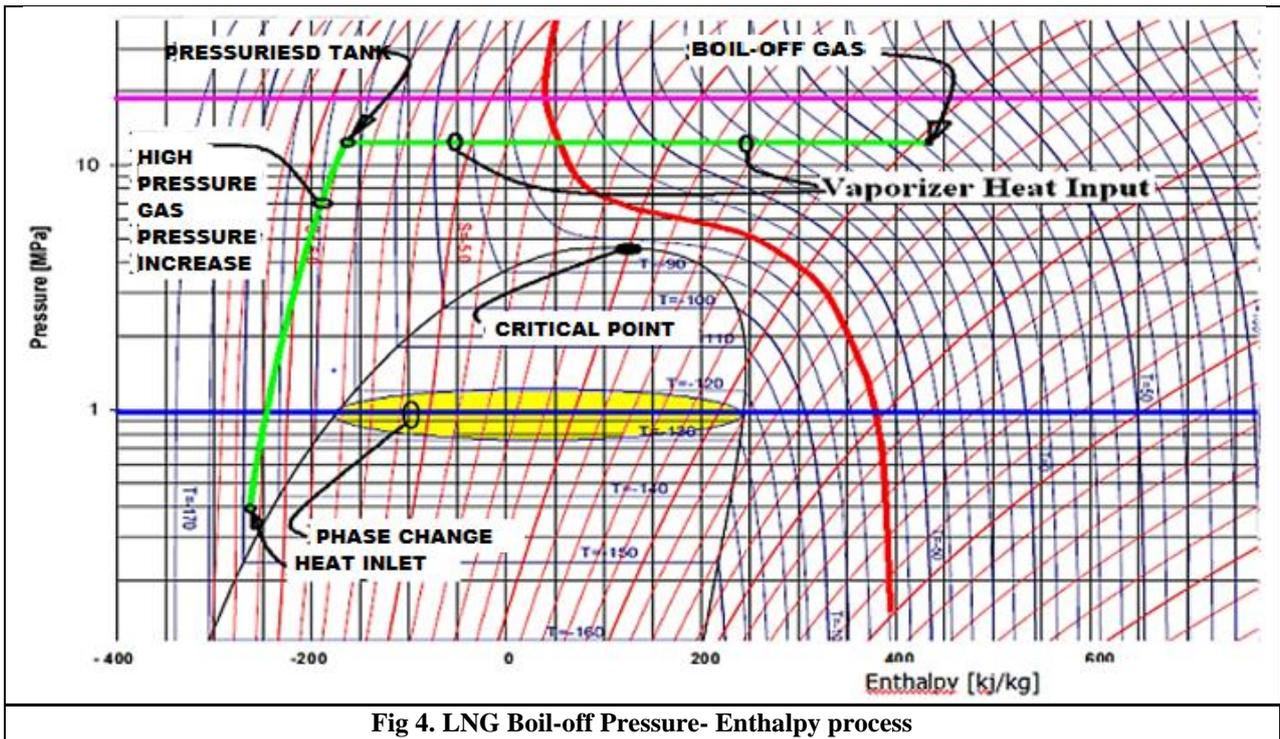
**Fig 4. LNG Boil-off Pressure- Enthalpy process**
