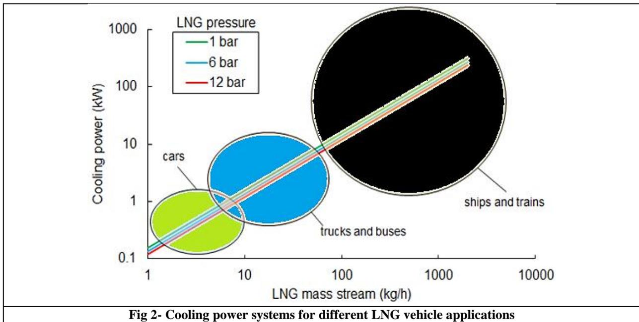
Fig 2- Cooling power systems for different LNG vehicle applications
