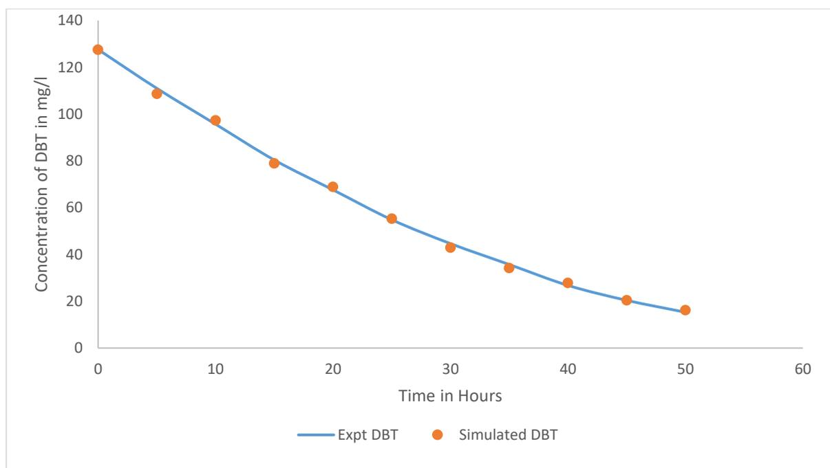
**Figure 6 Experimental and Simulated Data Plot of Concentration of DBT versus Time using Coated Bacterium**
