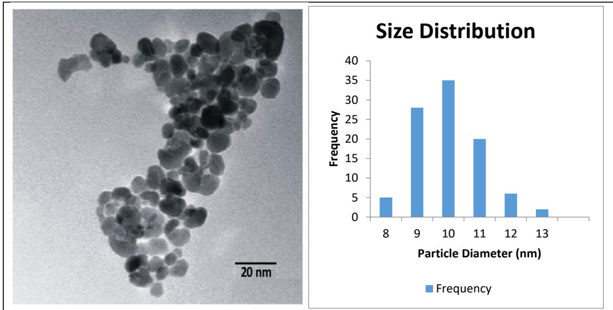
**Figure 1 TEM Image and Particle Size Distribution of the Synthesized Magnetite**
