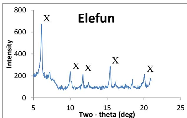
**Figure 9: XRD patterns for crystallized product at 6 hours**
