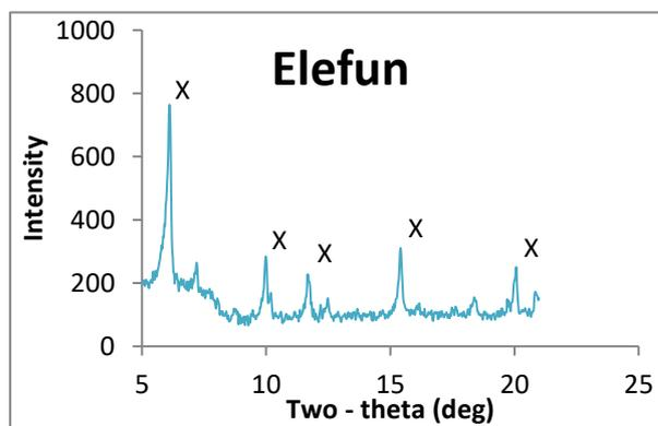
**Figure 10: XRD patterns for crystallized product at 12 hours**
