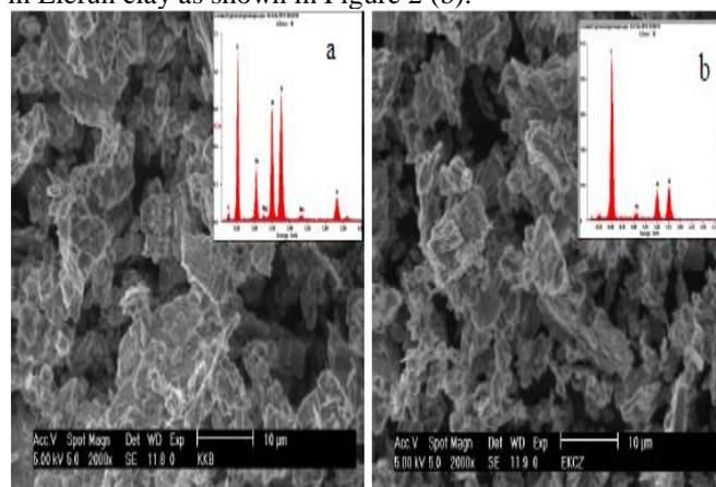
Figure 2: SEM and EDX for raw Kankara (a) and Elefun (b) kaolinite clay.
