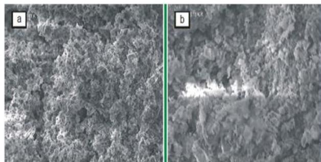
**Figure 4: SEM images for calcined Kankara (a) and Elefun (b) kaolinite clay.**
