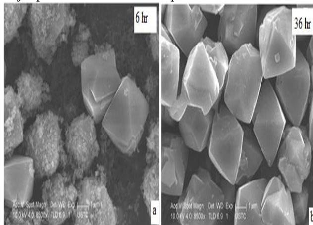
**Figure 13: SEM images for Kankara based NaX zeolite crystallized for 6hr and 36hr**
