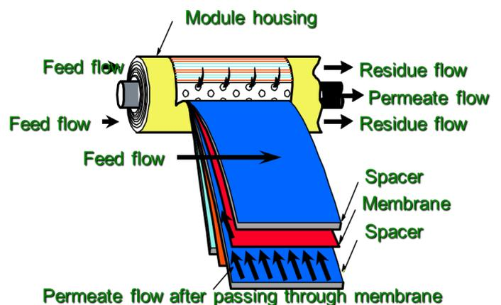
**Figure 1: Spiral wound membrane module;**( Source: MTR Inc, *Aquilo Gas Separation* )
