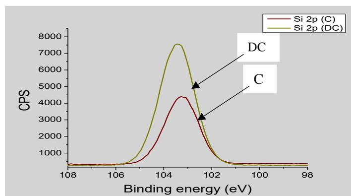
Figure 3: XPS Spectra of Si 2p of both clay and the dealuminated samples
