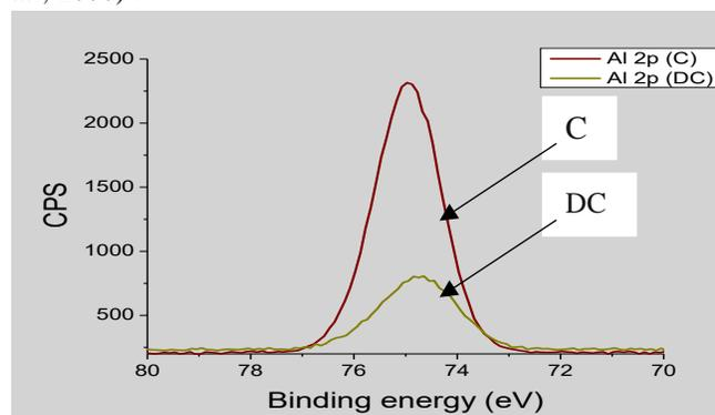
Figure2: XPS Spectra of Al 2p of clay and the dealuminated samples
