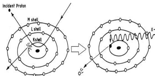
Fig 3 Basic Principle of PIXE analysis
